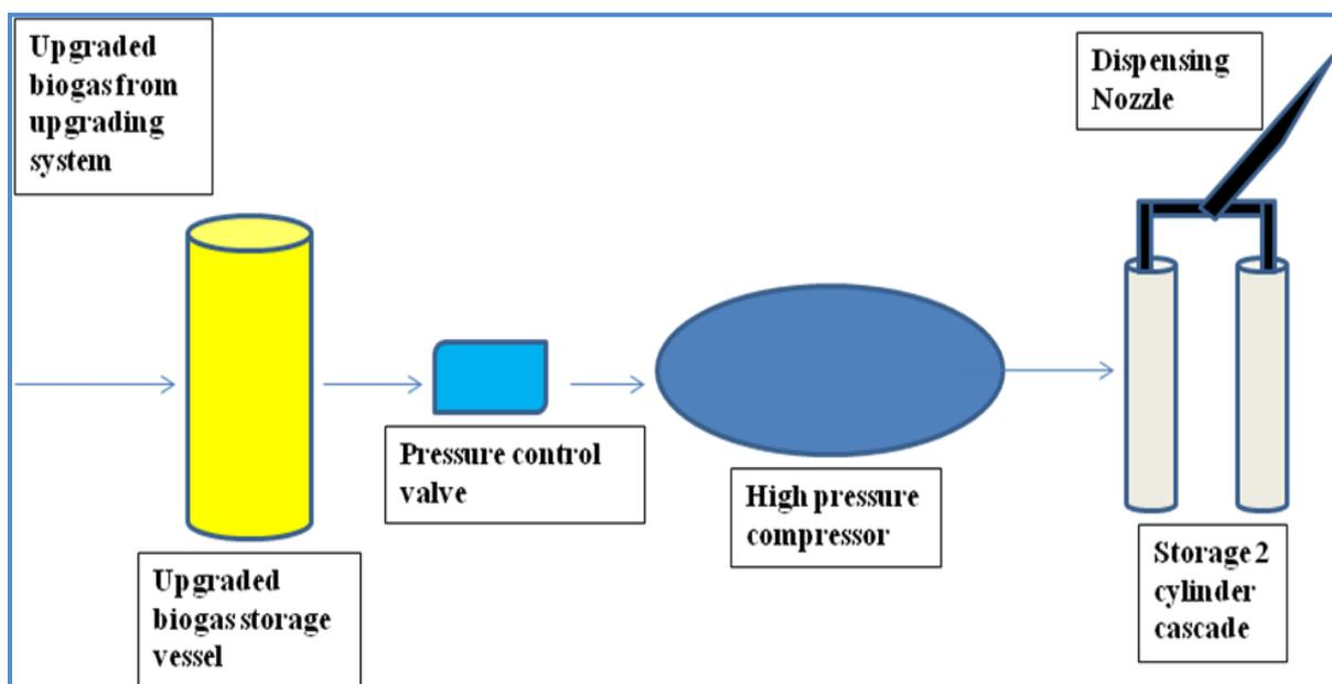
**Figure 16.** Upgraded biogas bottling system (Source: Authors)
