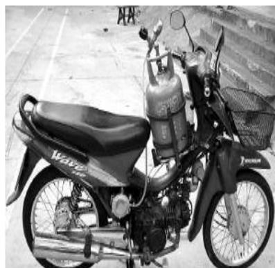
c) Motor-cycle run on LPG
