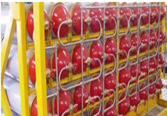
a) Cascade of CNG cylinders (*Source: <http://www.ramacylinders.in/cascade.html>*)
