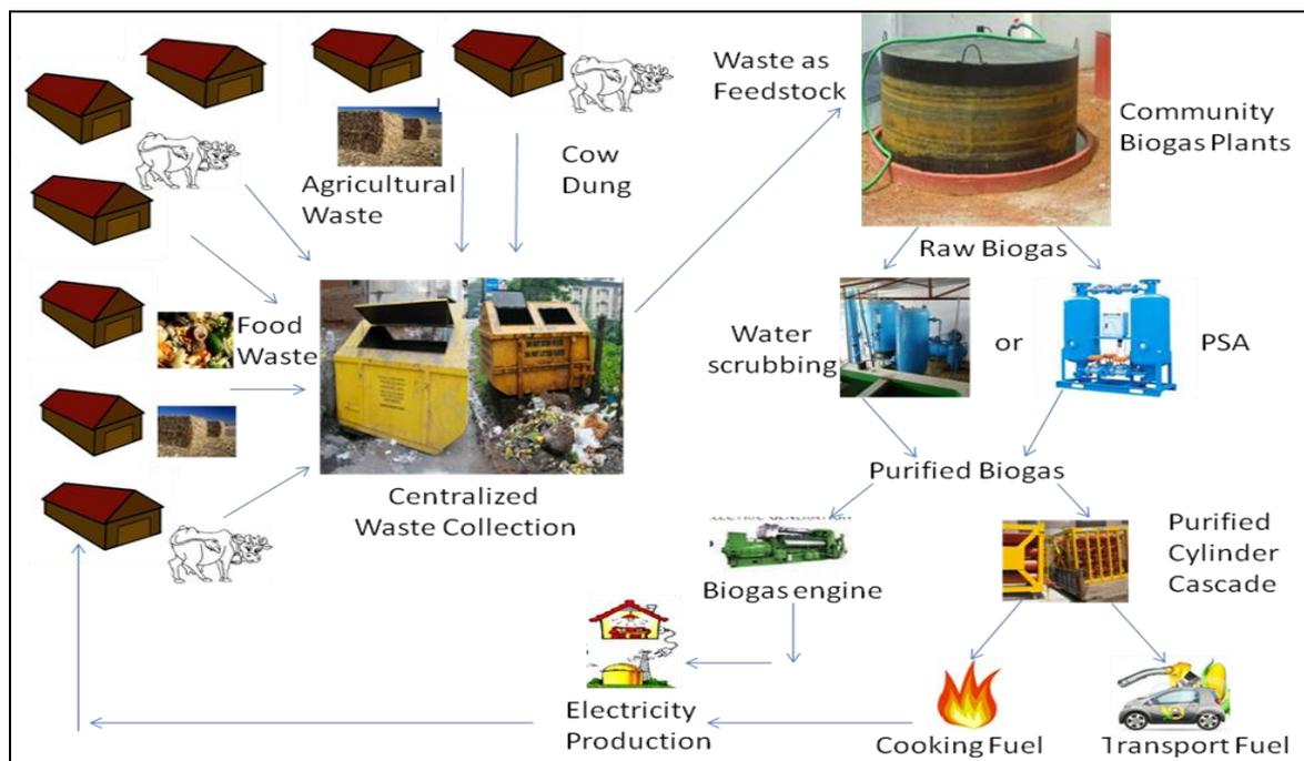
**Figure 32.** Schematic diagram of Biogas Entrepreneurship Model I (Source: Author).
