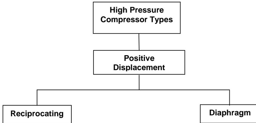
**Figure 17.** Types of High Pressure Natural Gas Compressors (*Source: Authors*)
