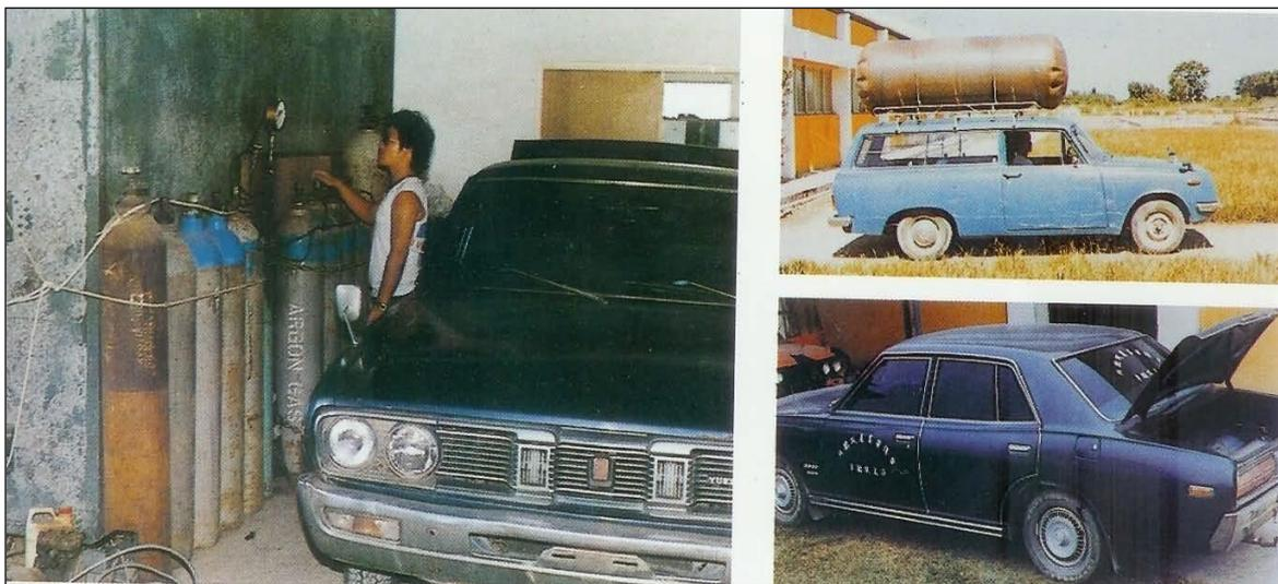
**Figure 11:** Biogas bottling and utilisation in vehicles in Taiwan (Source: Su J.J., 2011)
