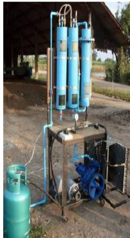
d) Biogas purification system
