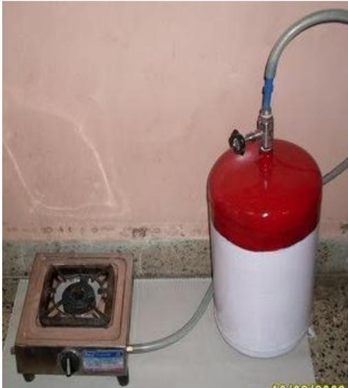
**Figure 2.** Bottled biogas used as a cooking fuel
