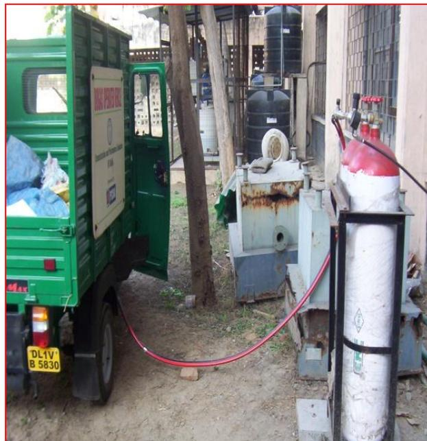
Upgraded biogas being dispensed into biogas vehicle
