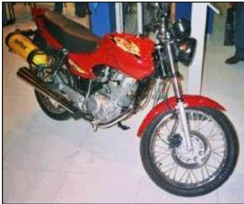
**Figure 7.** Biogas Motorcycle (Source: <http://www.inforse.org/europe/dieret/altfuels/biogas.htm>)
