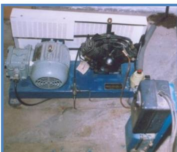
**Figure 20.** Small-scale high pressure gas compressor at IIT Delhi (Old) (*Source: Kapdi S.S, 2006*)
