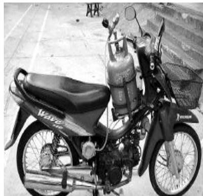
c) Motor-cycle run on LPG
