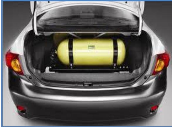
**Figure 14.** Car with CNG conversion kit (Source: <http://naturalgasconversion.net/>)
