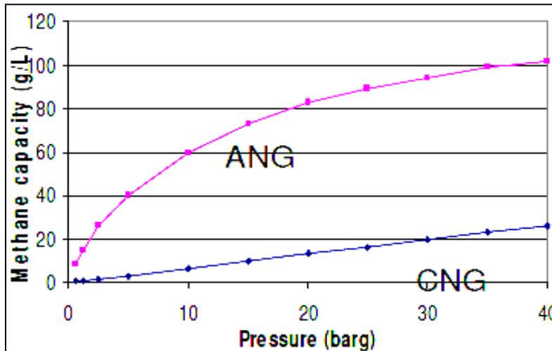
**Figure 27.** Methane storage capacity in CNG and ANG cylinders
