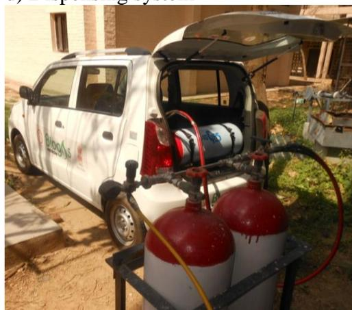
**Figure 31.** Simple low cost upgraded biogas dispensing system - demonstration system at IIT Delhi (Source: Authors)
