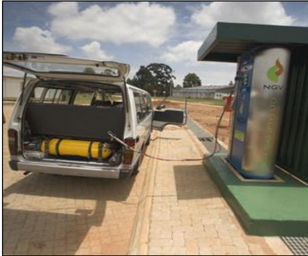
**Figure 13.** A dispensing station for demonstration purposes on a landfill site near OR Tambo International airport
