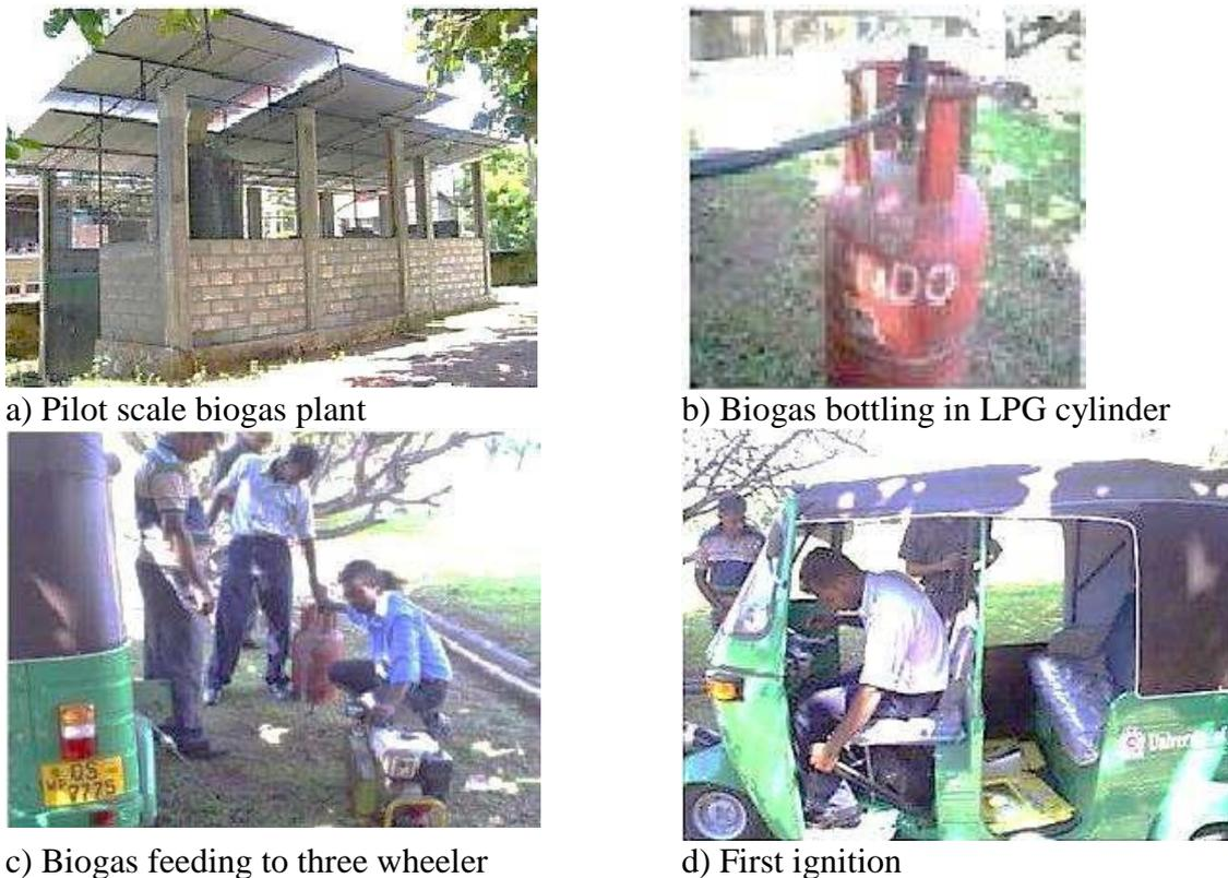
**Figure 9.** Pilot scale demonstration of biogas as a transport fuel at University of Moratuwa (Source: Alwis, 2012)
