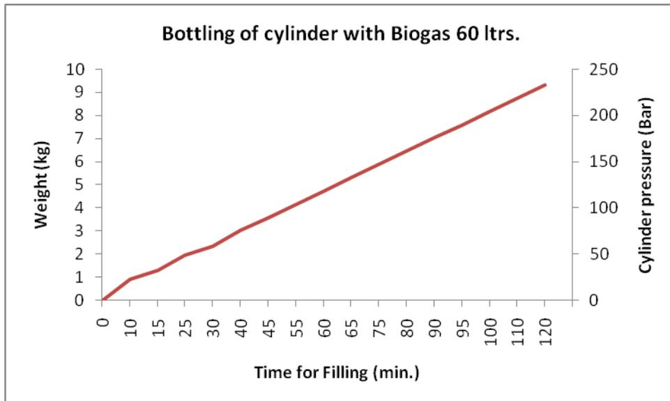
**Figure 26.** Graph showing the amount of upgraded biogas filled in 60-litre CNG cylinder
