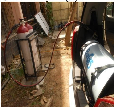
c) and d) upgraded biogas dispensing system being used to fill biogas vehicle
