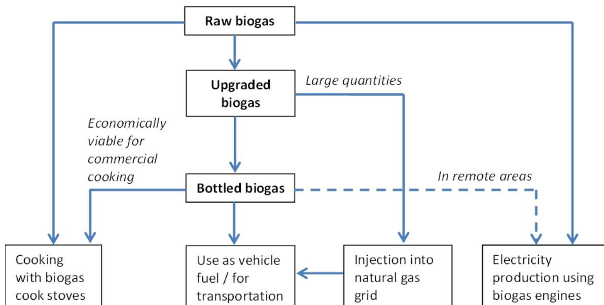
**Figure 1.** Different uses of biogas (Source: Authors)
