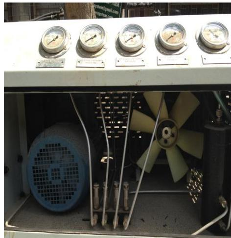
**Figure 21.** Newly procured high pressure small-scale compressor at IIT Delhi (*Source: Authors*)
